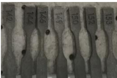
Figure 7 - Tensiles that were in contact with ATF Steering Fluid in Test 1- Type V
