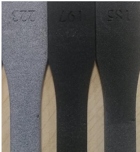
Figure 9 – Baseline, antifreeze-tested, brake fluid -tested tensiles after climatic chamber
