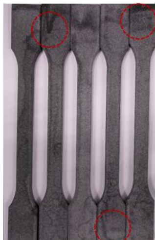
Figure 14: Type I samples after sterilization with Autoclave with visible marks.
